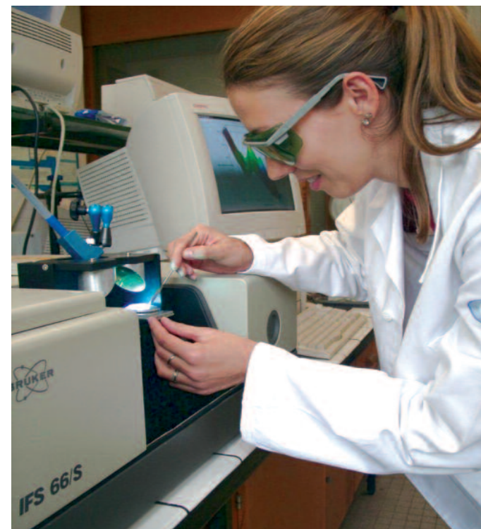
Kinetics studies of photopolymerization reaction by using Real Time FT-IR Spectroscopy
